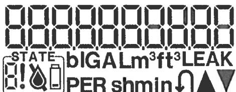
The water meter is fitted with an in-built LCD Display. 10 digits are available for Index display. Units available in European norm or American norm: m<sup>3</sup>; ft<sup>3</sup>; L, GAL, m<sup>3</sup>, ft<sup>3</sup>, L, per hour, minute or second.
